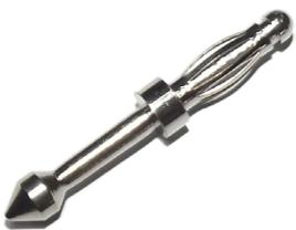
Ukuran : Poros steker diameter 4 mm, diameter ujung poros 4,5 mm, panjang 38 mm. Steker 4 mm, dilengkapi spring hull divernikel, diameter ujung poros 4,5 mm.
